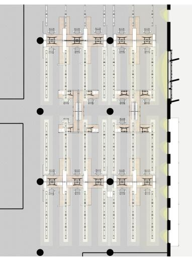
A smarter lighting design will help to provide even adequate lighting throughout the day, without over exposing those by the window or leaving others in the dark. Having lights running parallel to the exterior wall and set to different controls will allow for artificial lighting to be used by the window only when the sunlight in not sufficient.
