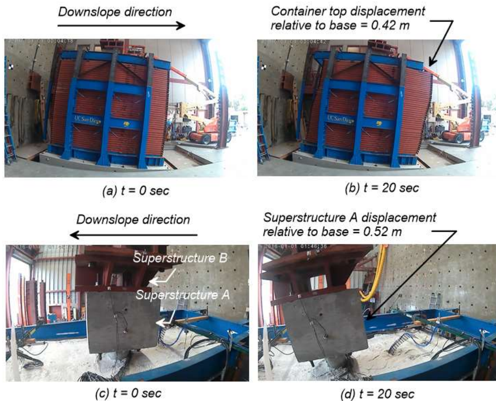
Figure 8. Side and top views of the model at the beginning (a,c) and end of the test (b,d).
