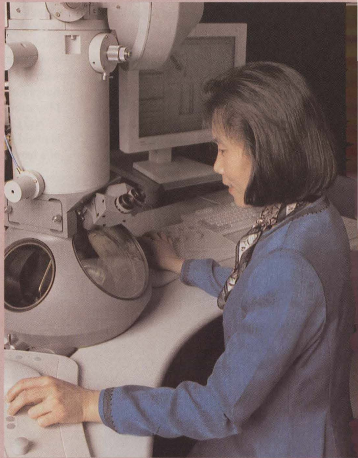
Jun Jiao, a director of the Nanoscience Center, uses the new transmission electron microscope for looking at nanotubes, hollow tubes of carbon atoms.
