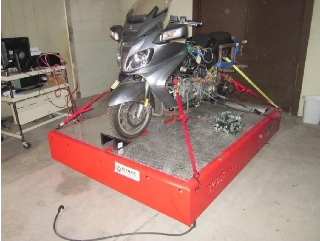
Figure 1.16 – The dynamometer with the Green Lite vehicle in the OIT dynamometer test room
