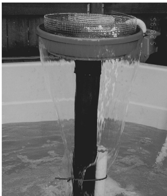
FIG. 3. Experimental fountain showing contraction of the water sheet with a height of about 70 cm.
