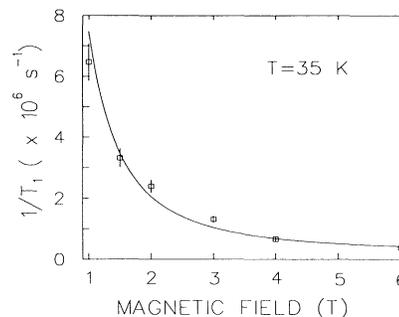
FIG. 2. The magnetic field dependence of  $T_1^{-1}$  in  $Rb_3C_{60}$ . The solid curve is a fit to the muonium spin exchange model (see text).
