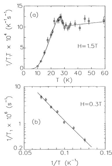
FIG. 3. (a)  $(T_1 T)^{-1}$  in  $Rb_3C_{60}$  at a magnetic field of 1.5 T. The solid curve is a fit to the theory of Hebel and Slichter with a broadened density of states. (b) Arrhenius plot of  $T_1^{-1}$  in a magnetic field of 0.3 T.
