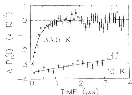
FIG. 1. Muon spin relaxation of endohedral muonium in  $Rb_3C_{60}$  above and below  $T_c$  in a longitudinal magnetic field of 1.5 T. The  $y$  axis is the muon spin polarization  $P_z(t)$  of muonium multiplied by an experimental constant  $A$  which is negative for our geometry.
