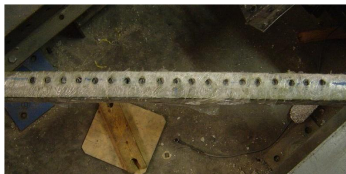
Figure 2.2: Modified Section of a Specimen Retrofitted with a 3-inch x 3-inch FRP Tube.
