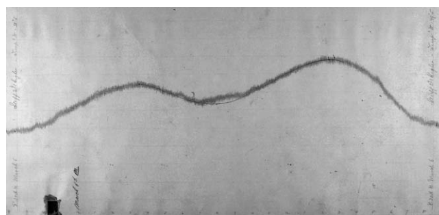
Figure 4. Marigram from 5 March 1862, from San Francisco, California. Nontidal fluctuations are evident and required interpolation by the tabulator to estimate the astronomical low water (see interpolation line and low-water point). The thick pencil line indicates atypical, short (<1 minute) fluctuations caused by a stilling well problem or by dock vibrations after moving the gauge to a new gauge house, which was necessitated by the severe storms of December 1861 to February 1862.
