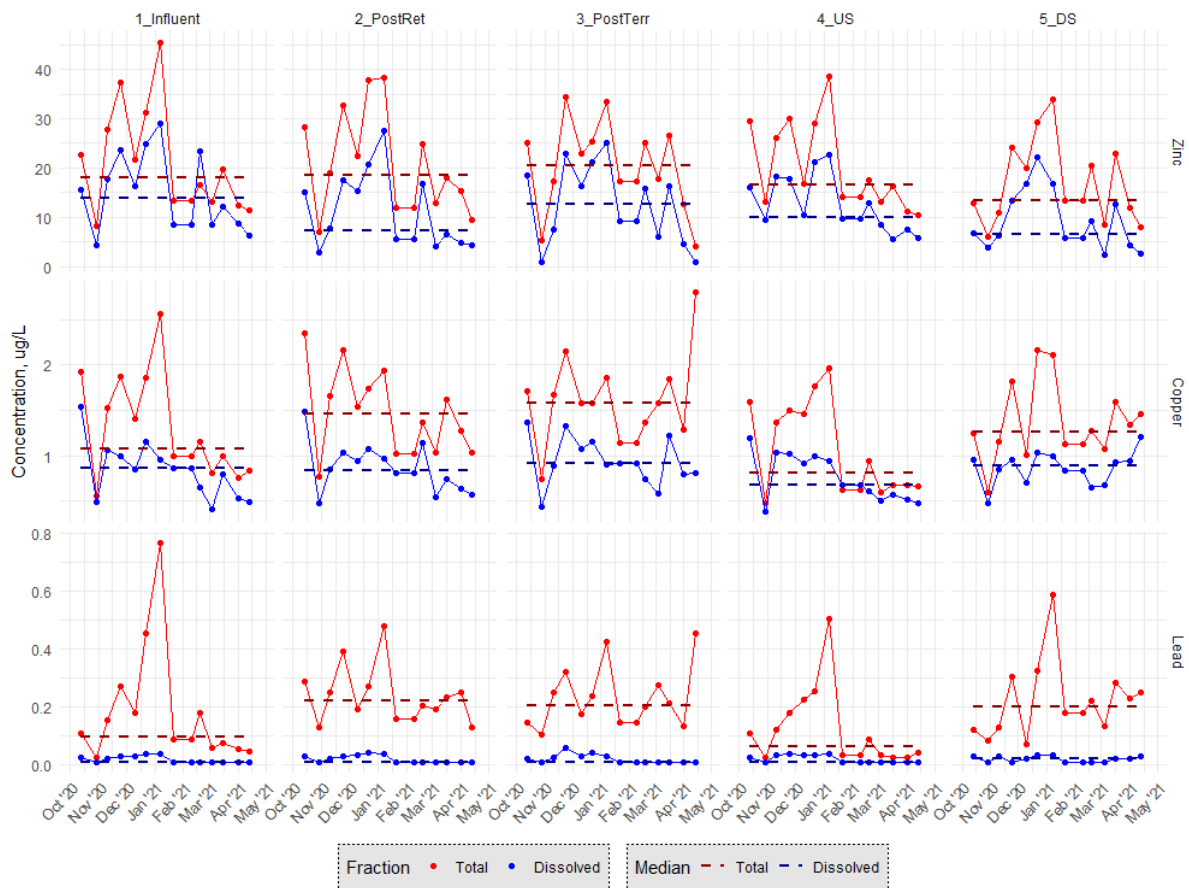
Figure 25. Total and Dissolved metals (Zinc, Copper, and Lead) concentrations, divided by monitoring point, and respective study-wide median concentrations for each metal and fraction of metal.
