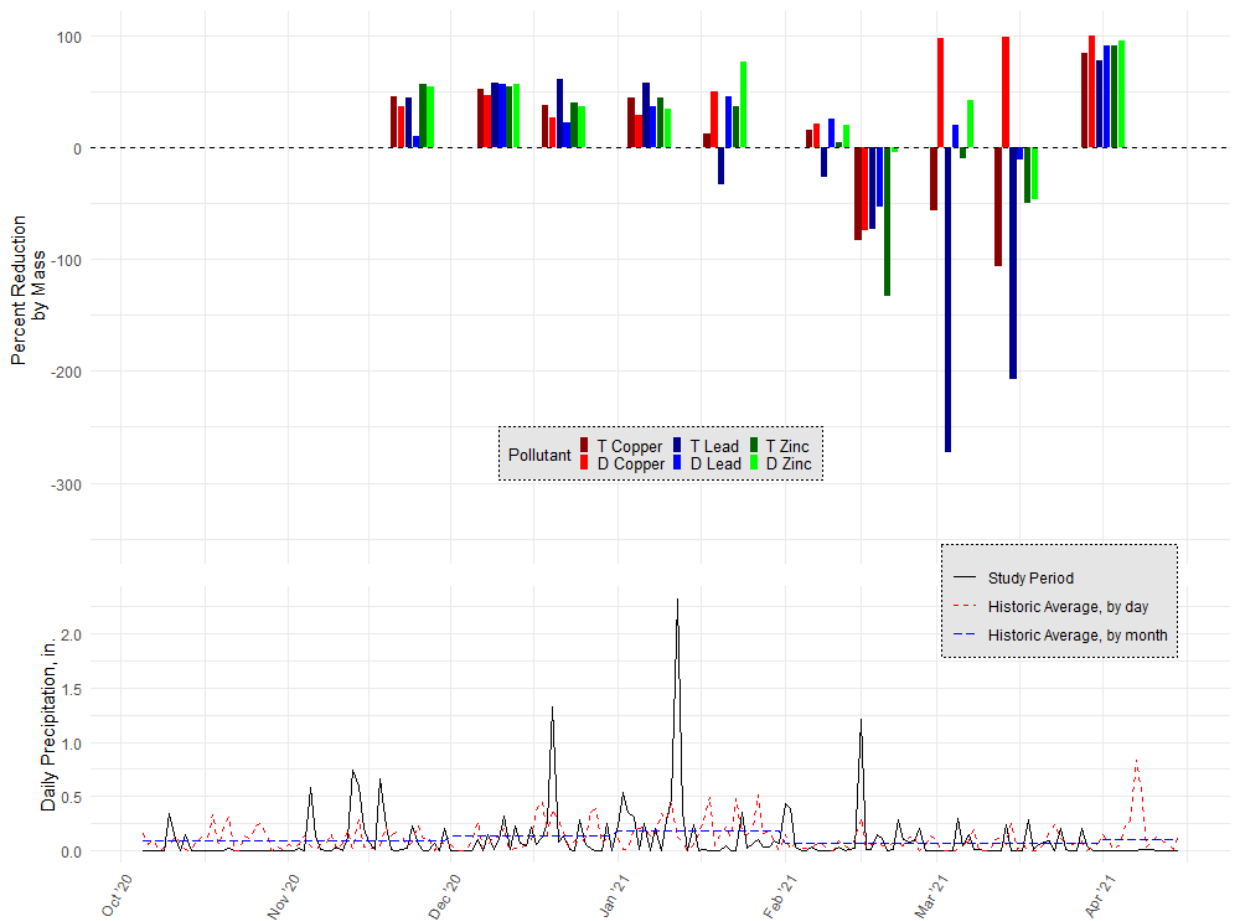
Figure 28. Mass-based reductions for metals (“T”= total, “D”= dissolved) between Site 1 and Site 3 of the CW compared to a nearby precipitation gage across the study period. Historic precipitation record from September 2017-September 2020. Positive Reductions imply the mass or concentration decreased across the CW (i.e., from Site 1 to Site 3). Negative Reductions imply an increase.
