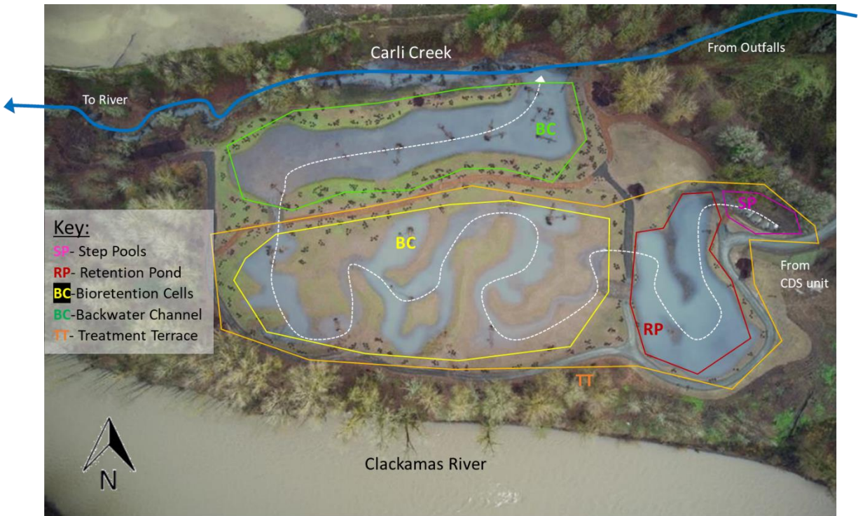
Figure 9. Aerial map of the treatment terrace showing separate regions of the treatment terrace (“TT”), Carli Creek, and the Clackamas River. SP=step pool, RP=retention pond, BR=bioretention cells, BW=backwater channel.
