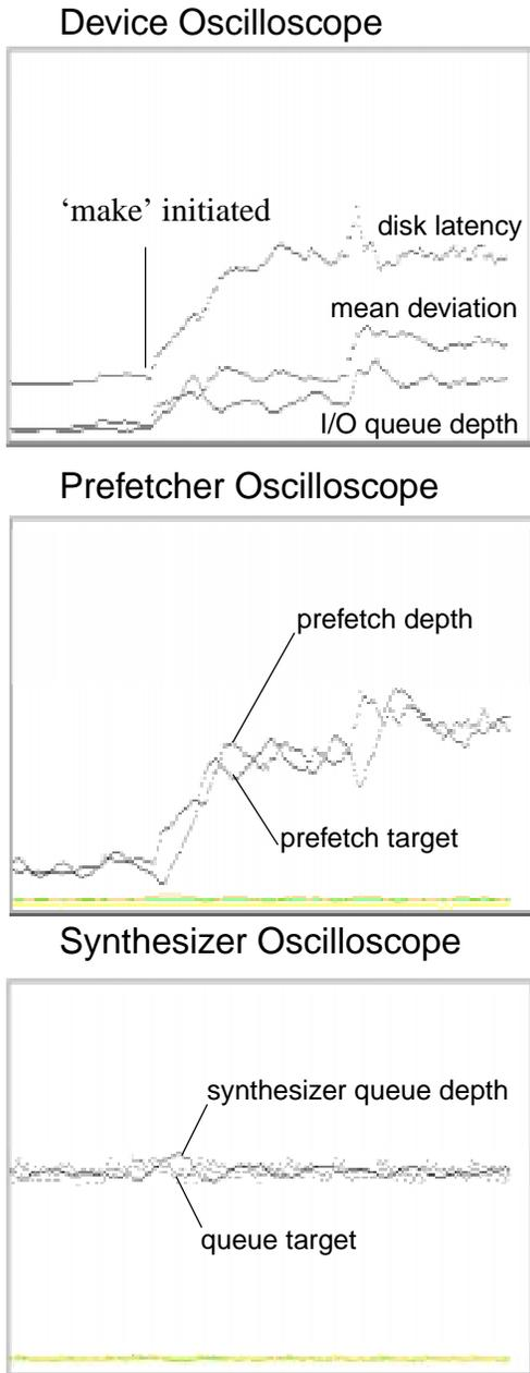
**Figure 5: Adapting to I/O contention.** These oscilloscope snapshots depict the I/O status of various levels of the system. A 'make' was initiated at the point indicated in the top graph, which introduced contention to the disk, resulting in increased I/O latencies. As expected, the prefetcher adapts to the load, hiding it from the synthesizer.
