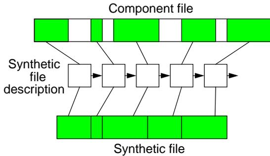
**Figure 1: Synthetic file description.** Synthetic files describe complex access patterns to component files. An application describes its accesses in domain-specific terms. This description is translated into an assembly of data units for lower layers of the system.
