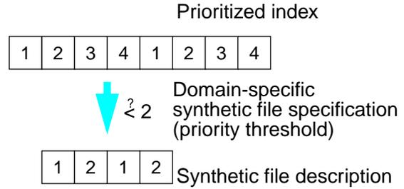
**Figure 4: Domain-specific synthetic file specification for adaptive video streaming.** The adaptive media stream separates quality axes into separate data units. The adaptation policy labels each unit with its component’s priority. The synthetic file can be expressed with a simple priority threshold, which is interpreted by the synthesizer to create a synthetic file
