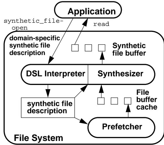
**Figure 3:** The interactions between an application, the file synthesizer and the prefetcher. The synthesizer interprets the domain-specific synthetic file description to determine the data to fetch, and translates it into the description needed by the prefetcher.
