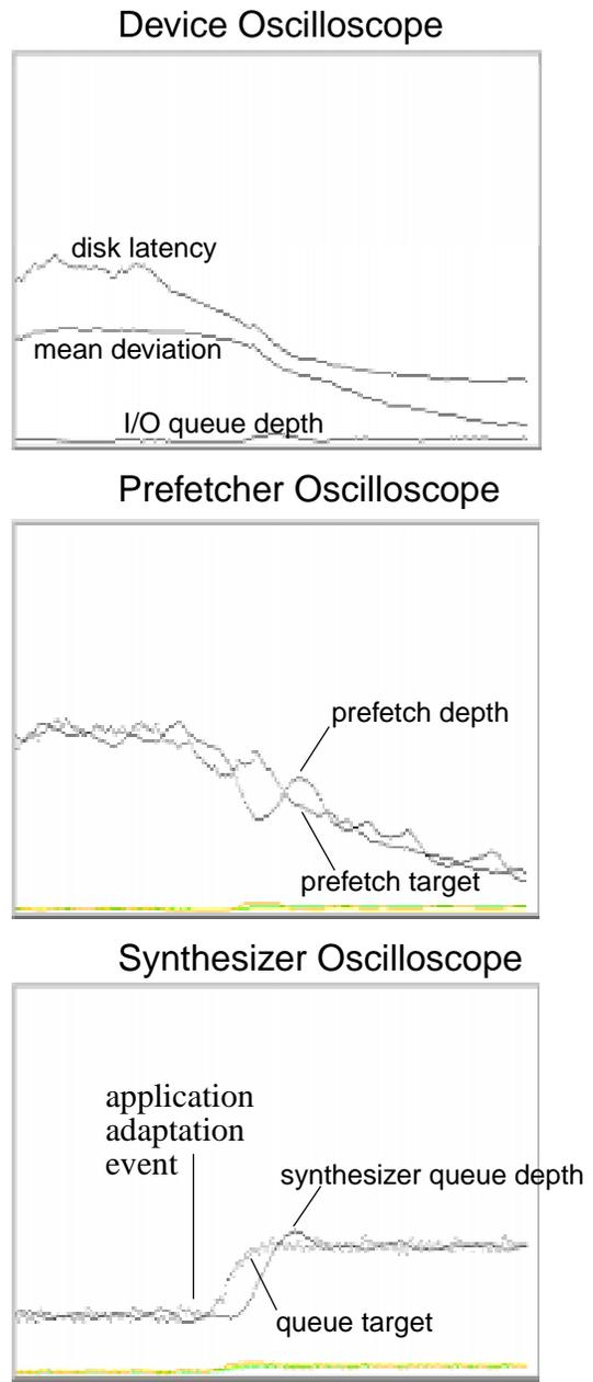
**Figure 6: Adapting to application-level adaptation.** This set of oscilloscope snapshots show the system reacting to an application adaptation. The application has adapted to improve quality. The bottom chart shows the synthesizer reacting to the application by increasing its queue depth to match the application's higher rate. The improved sequentiality of the higher data rate stream results in *lower* I/O latencies and corresponding lower prefetch depth.
