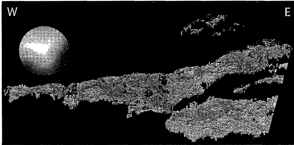
Figure 12: Example of a Coltop 3D view of the point cloud. The color of each point of the scan is given by the orientation (using the pole) of the surface at this point in the colour wheel. The view is from a point at the South of the cliff.
