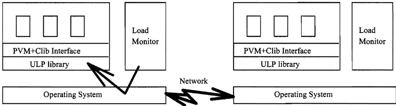
Figure 5: Software architecture of an ULP based system
