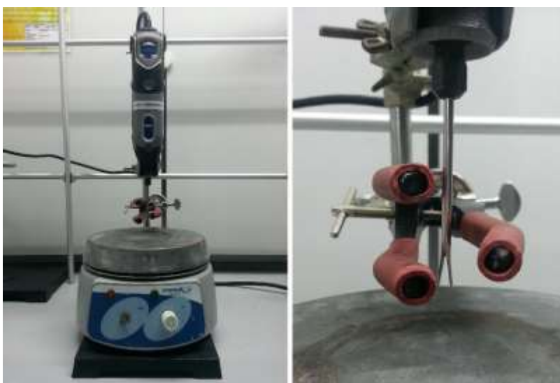
Figure 2.2: Custom Homogenizer. Outfitted Dremel on its stand (left). 1/8th SS mixing bit (right).
