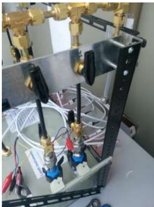
Figure 3.2: Fully Assembled Swagelok Cell connected to the oxygen supply system.
