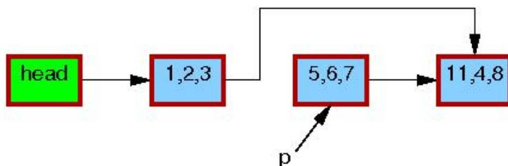
Please note that readers are not permitted to maintain references to element `5,6,7` after exiting from their RCU read-side critical sections. Therefore, once the `synchronize_rcu()` on line 4 completes, so that all pre-existing readers are guaranteed to have completed, there can be no more readers referencing this element, as indicated by its black border below. We are thus back to a single version of the list.
