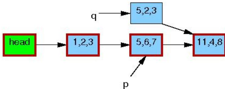
Now, line 5 does the replacement, so that the new element is finally visible to readers. At this point, as shown below, we have two versions of the list. Pre-existing readers might see the 5,6,7 element, but new readers will instead see the 5,2,3 element. But any given reader is guaranteed to see some well-defined list.
