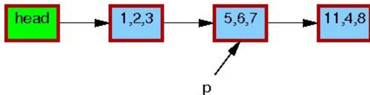
As before, the triples in each element represent the values of fields  $a$ ,  $b$ , and  $c$ , respectively. The red borders on each element indicate that readers might be holding references to them, and because readers do not synchronize directly with updaters, readers might run concurrently with this entire replacement process. Please note that we again omit the backwards pointers and the link from the tail of the list to the head for clarity.
