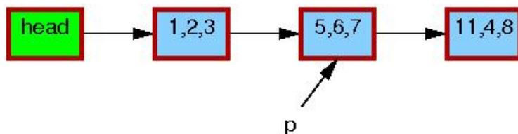
The triples in each element represent the values of fields  $a$ ,  $b$ , and  $c$ , respectively. The red borders on each element indicate that readers might be holding references to them, and because readers do not synchronize directly with updaters, readers might run concurrently with this entire replacement process. Please note that we have omitted the backwards pointers and the link from the tail of the list to the head for clarity.
