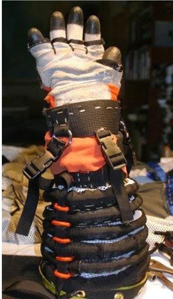
FIGURE 2. Finished Constant Volume Elbow Joint (left) and Joints Installed in Pressure Garment (right).
