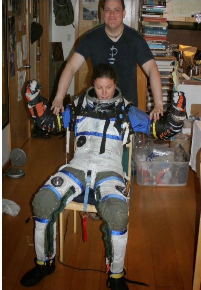
FIGURE 2. Finished Constant Volume Elbow Joint (left) and Joints Installed in Pressure Garment (right).
