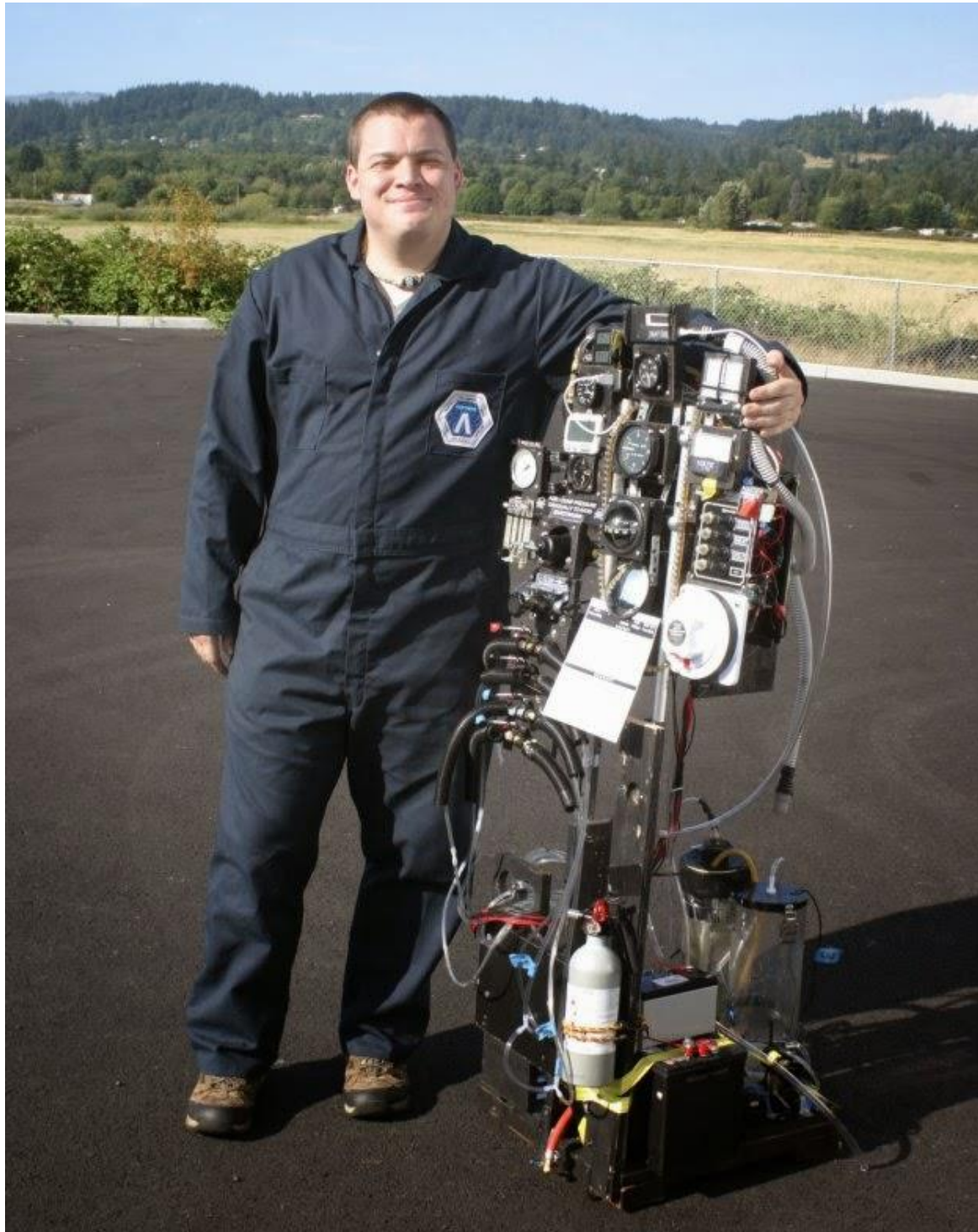
FIGURE 4. Pacific Spaceflight Crewmember AK Knapton With the Portable Life Support System (PLSS) Prepared for Use in Bell 206 Jet Ranger, Before Custom Fitting. SCUBA tank noted in Figure 3 not installed in this photo. This stripped-down PLSS manifestation was named 'Skeletor' as it was significantly reduced in bulk and weight from prior builds.
