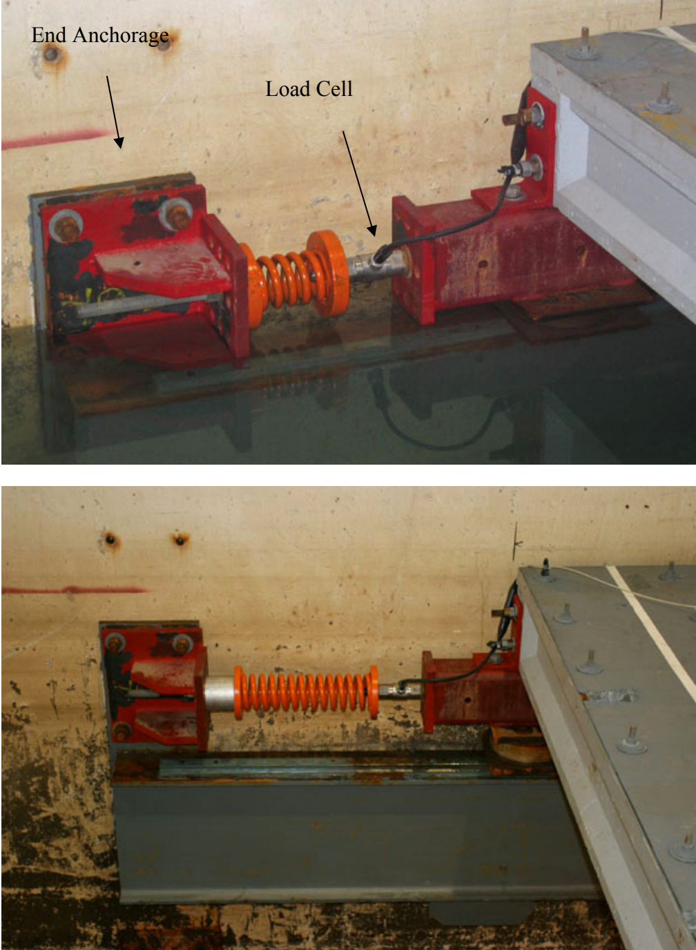
Figure 3.7. Photos of stiff (top photo) and soft (bottom photo) springs installed with horizontal load cell, LC2.
