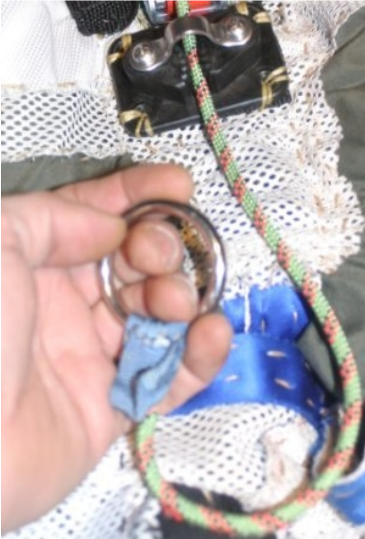
FIGURE 2. Sailing vessel spring-activated cam-action cleat used as helmet hold-down locking mechanism in test reported here.
