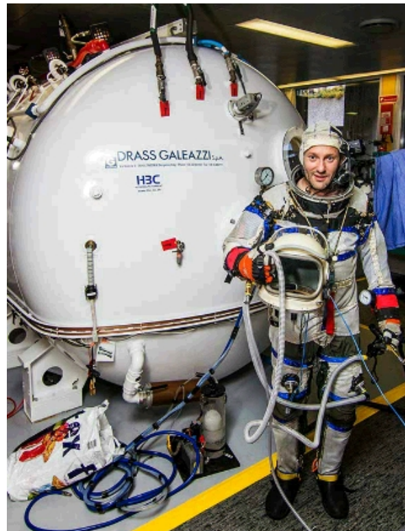
FIGURE 1. (A) Test Subject Standing Before the Trykkammer Wearing the Mark I ( Gagarin ) Pressure Garment. The flight coverall was not worn in this test; visible is the pressure restraint garment that covers the gas retention layer. (B) Test Subject (L) and Pressure Garment Operator (R) During Depressurization Test. Photos courtesy of Jev Olsen, Copenhagen Suborbitals.
