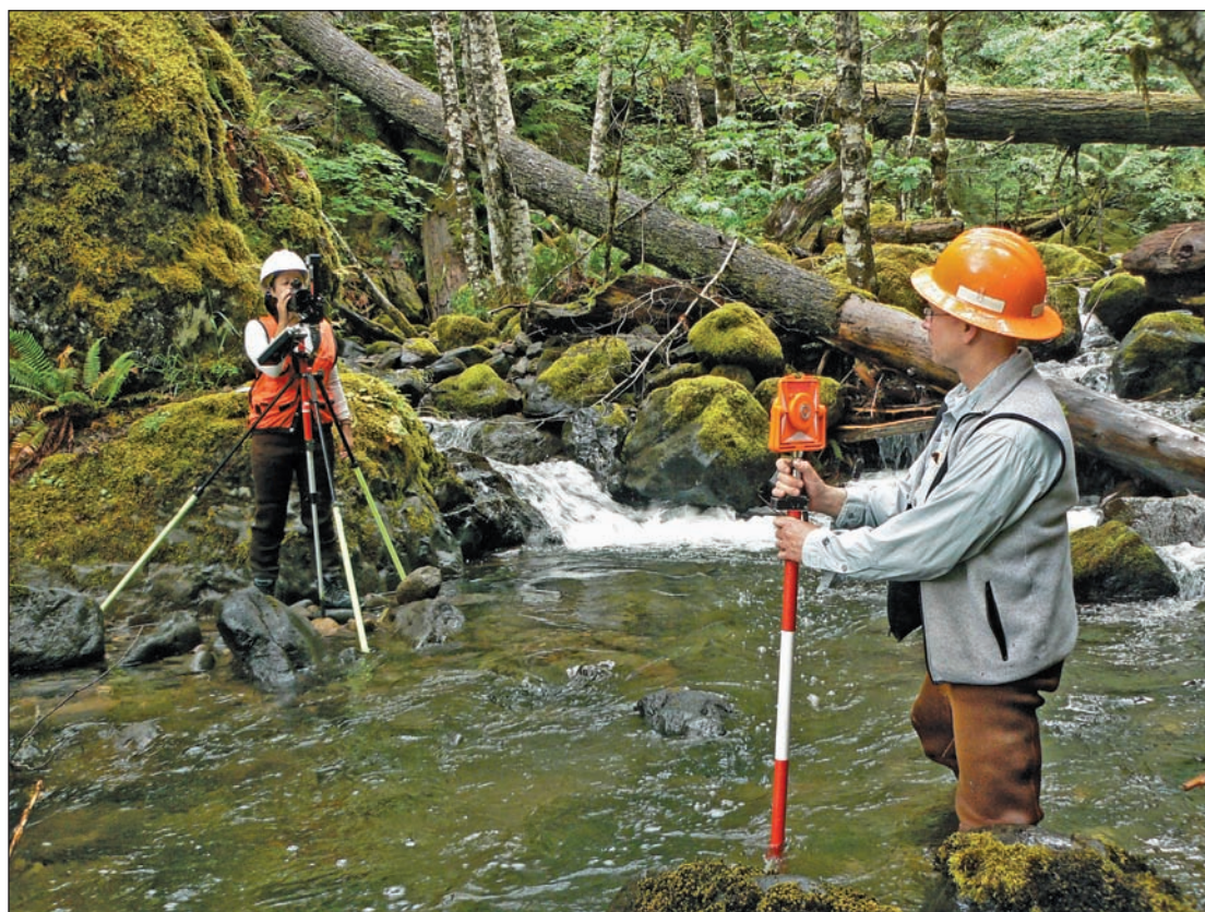
Figure 7—Bankfull width-to-depth ratios were calculated from cross-sectional profiles.
