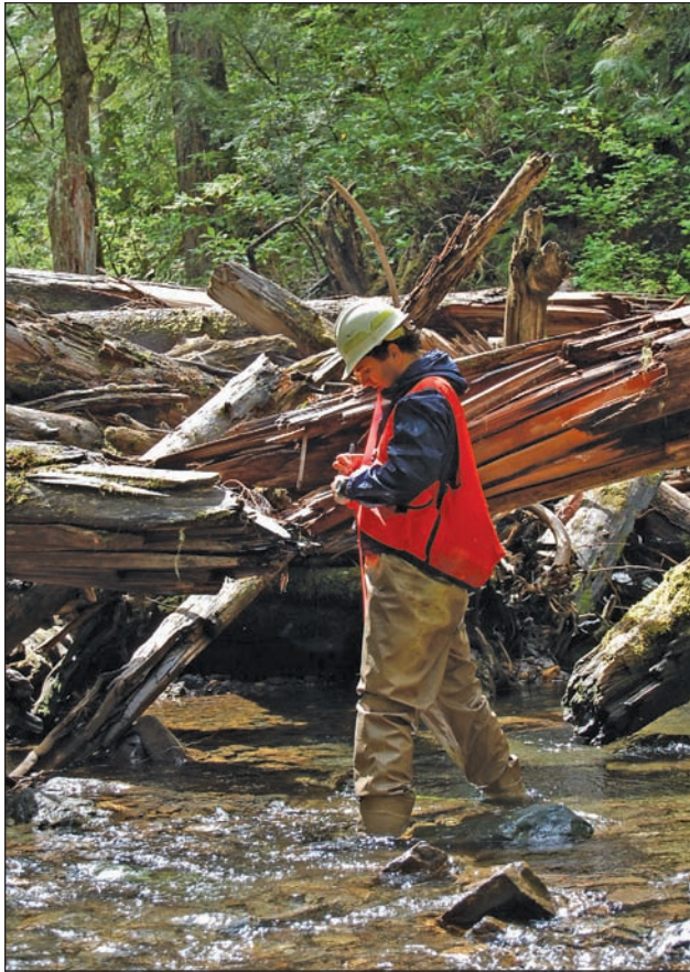
Figure 8—Large pieces of wood in the stream channel were counted in each sampled stream reach.
