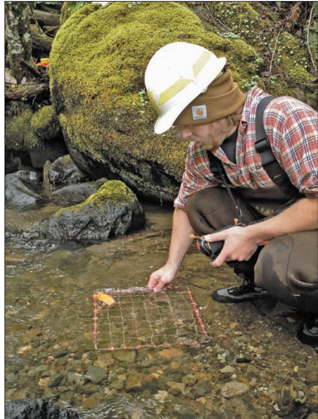
Figure 9—Fine sediment was measured at pool tail crests.
