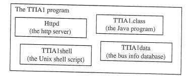
The TTIA1 program consists of an http server, a shell script, a Java program and a database. The http server is a large, fancy program and was available for use as a component of TTIA1 without needing modification. Though TTIA1 can't function without the http server, it's important to note that the server, unlike the other components, exists on the host computer separate from TTIA1 and is employed for many other purposes.
