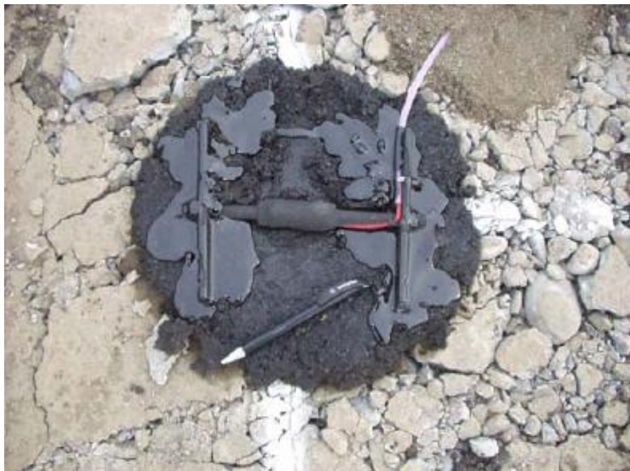
Figure 3.1: Close-up view of an ASG-152 strain gage.
