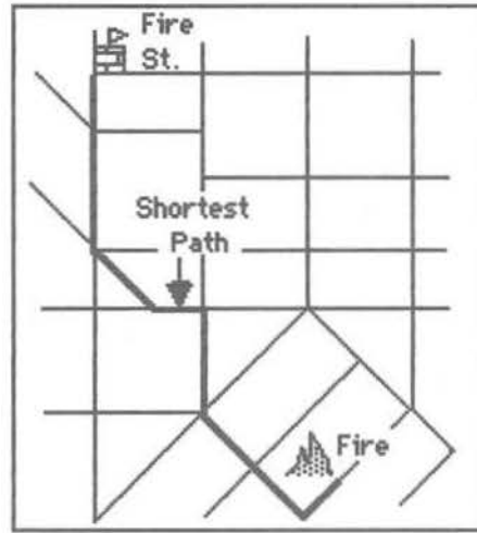
FIG. 3-The TIGER file allows one to do specialized operations, like determining the shortest path between an emergency and a responding emergency vehicle.
