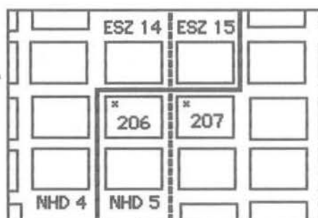
FIG. 2—In TIGER, individual blocks are maintained. This allows derivative files for larger districts. For example, blocks 206 and 207 are contained in the neighborhood NHD 5. Block 206 is contained in ESZ 14 and block 207 is contained in ESZ 15. Maintaining individual block units is the key to deriving multiple district files.
