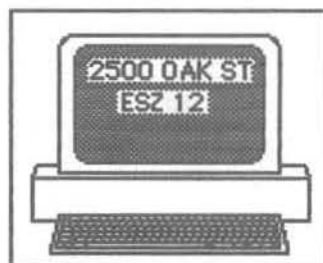
FIG. 1—E911 immediately displays a caller's address and emergency service zone on the dispatcher's screen.
