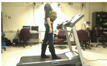
Figure 1: Representative image of a subject wearing a loaded ammunition pack while walking on the laboratory treadmill. There was no slope to the walking surface for this particular study ( 0^\circ incline setting). Note that the pack load is distributed about the subject's mid-section with front-load pockets, near their body center of mass (cm Body).
