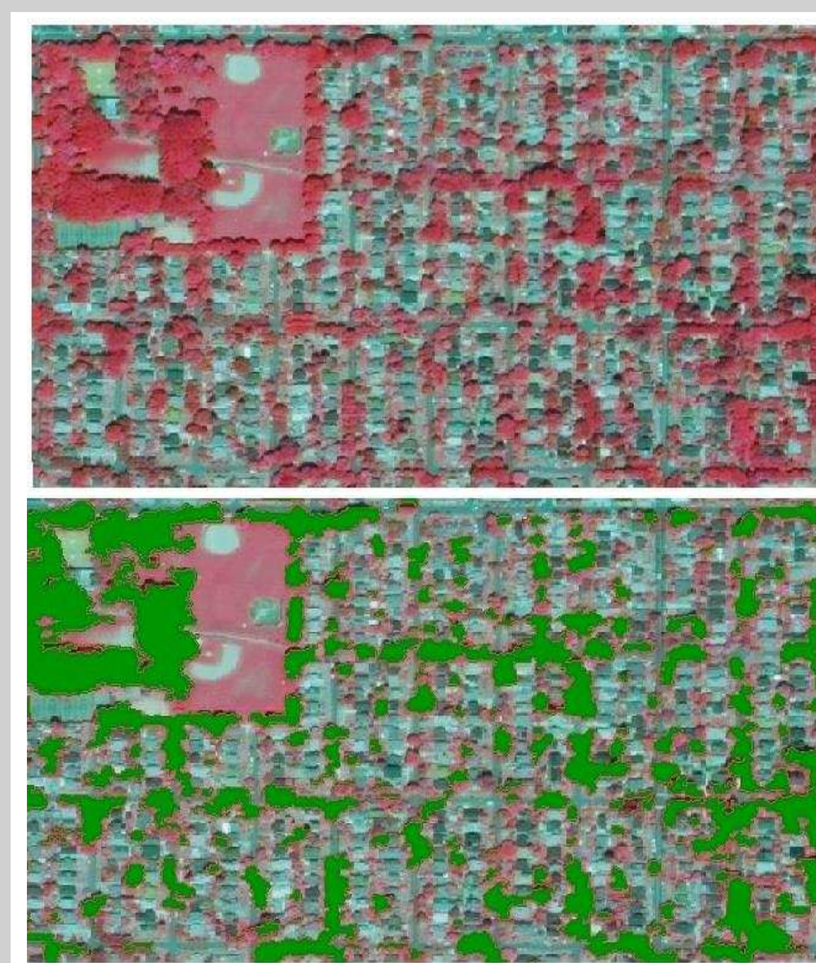
Figure 4. Example of canopy cover analysis using NIR imagery
