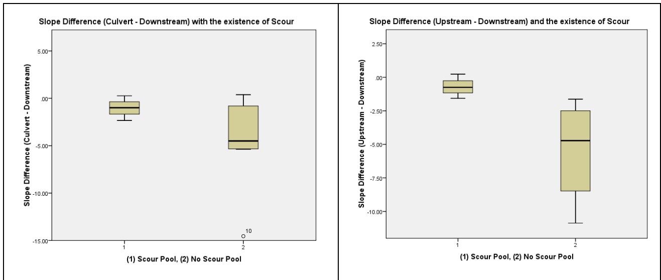
Figure 5.8: Slope Differentials vs. scour
