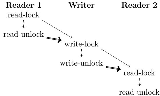
Figure 3.15: Orderings required for reader-writer lock semantics.
