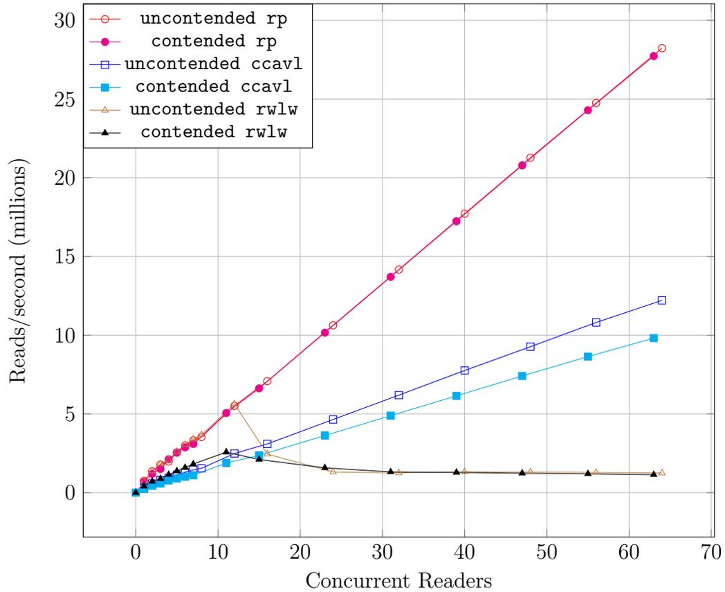
Figure 4.10: Contended and uncontended read performance of 64 node red-black tree using a variety of synchronization techniques.
