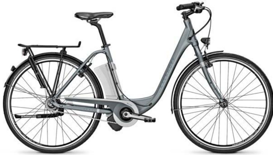
Figure 2-2: Kalkhoff Sahel I8—a modern power-assisted bicycle (PAB) or pedelec. Image source: Kalkhoff-Bikes.com
