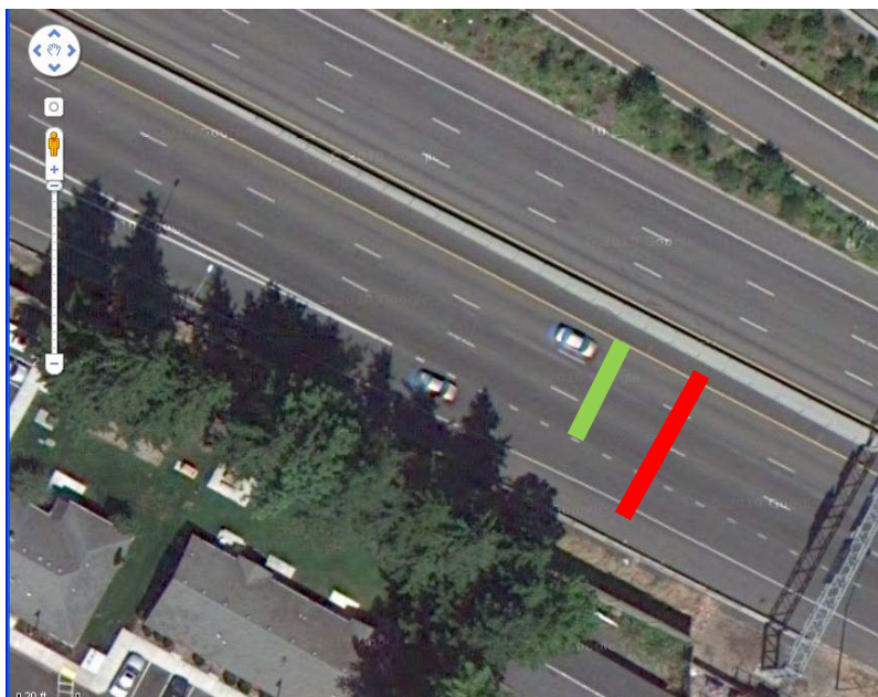
Figure 17. Difference in number of lanes. PORTAL (green line) counts three freeway lanes where the imported VISUM/NAVTEQ network (red line) has four.
