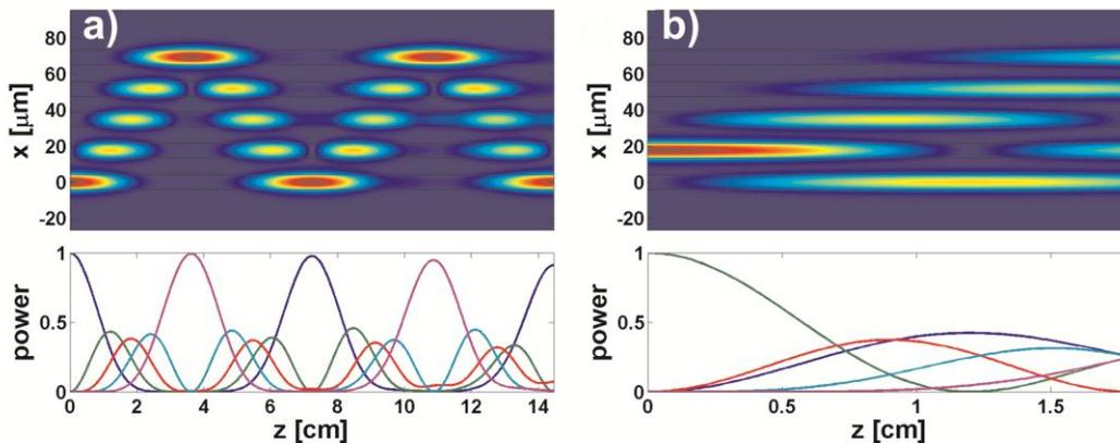
**Fig. 1** Numerical simulation of a commensurate 5-waveguide array with a) the input state  $(1, 0, 0, 0)$  and arbitrary length, b) the input state  $(0, 1, 0, 0)$  and the length that renders equal 1x4 coupler.
