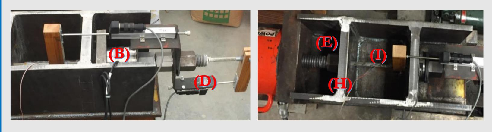
(A): Hollow-core ram (B): Load cell (C): LVDT-1 (D): LVDT-2 (E): Hex nut
