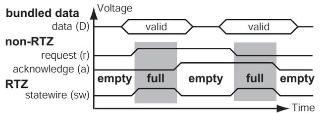
**Figure 3** Non-RTZ and RTZ two-phase handshake variants. By convention, data must be valid when the link is full, and may change only when the link is empty. In reality, data may be kited, as long as the values are valid when captured.
