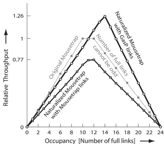
**Figure 8** Three canopy graphs for simulations of rings with 24 pipeline stages. The center graph with fewer data points is from simulation with an original Mousetrapped module. Naturalizing its links with the circuit of Figure 6(c) produces the lower graph. The increased number of logic gates costs performance. Using the link circuits of Figure 6(b) produces the upper graph, improving the original performance. These three 90nm simulations omit data latches and wire loads.
