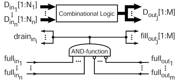
**Figure 7** Design sketch of a joint without stored state with  $n$  naturalized incoming and  $m$  naturalized outgoing links, where  $1 \leq i \leq n$  and  $1 \leq j \leq m$ . If data are just copied then  $D_{out_j}[1:M]$  is the concatenation of  $D_{in_1}[1:N_1]$  to  $D_{in_n}[1:N_n]$  and  $M = N_1 + \dots + N_n$  ( $N_1, \dots, N_n \geq 0$ ).
