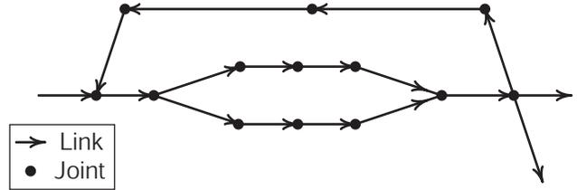
**Figure 1** A self-timed dataflow system with communication channels, called links, and flow control and data computation modules, called joints, can be viewed as a directed graph with data flowing in the direction indicated by the arrows.
