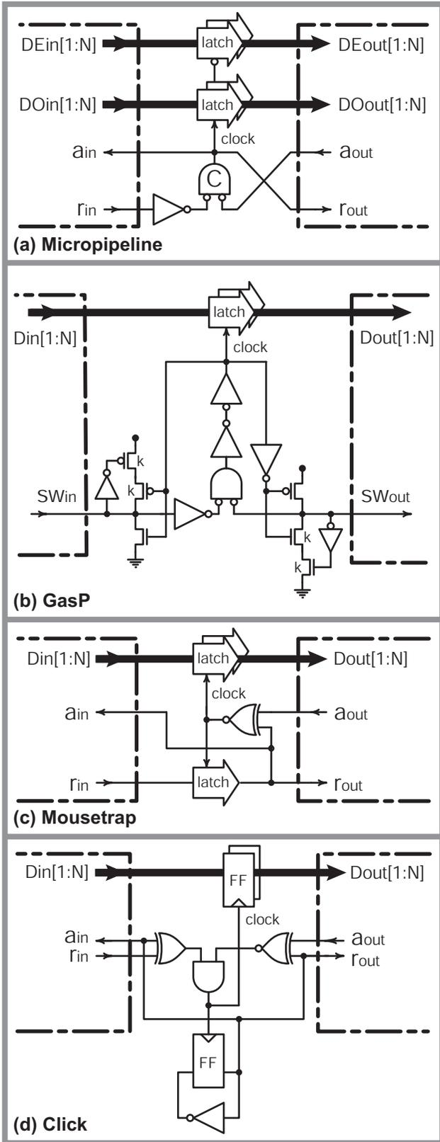
**Figure 2** Circuit designs for a single-input single-output FIFO module in each of the four bundled-data two-phase circuit families. The dashed lines mark the interface between the joint in the middle and the left-hand and right-hand links. Note that the joints hold all the logic for flow control and data computation — the links are “just wires.”
