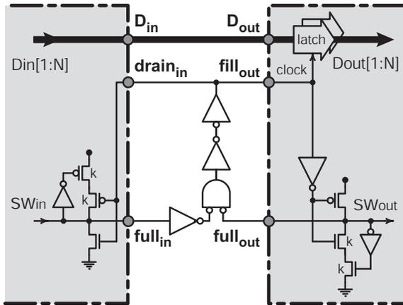
**Figure 4** Circuit re-design for the GasP FIFO module of Figure 2(b). The responsibility for capturing data has moved from the joint to the receiving link. Representing full or empty is now entirely in the links. We colored “link logic” grey, reserving the white center for the simplified joint.
