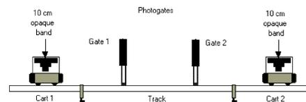
Figure 1: Diagram of a typical photogate-based experiment [3].
