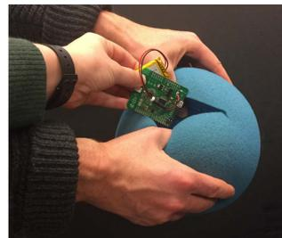
Figure 3: Insertion of an position tracking device into a foam ball.
