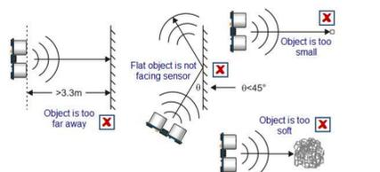
Figure 2: Unusable configurations for ultrasound sensors [4].
