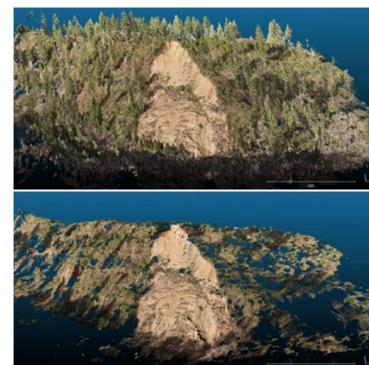
Figure 9: Above, Cedar Creek full point cloud. Below, ground-only point cloud after CSF algorithm.
