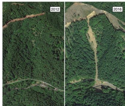
Figure 7: Wilson River landslide imagery from Google Earth Pro shows active roadbuilding in 2012 and subsequent landslide in 2016.
