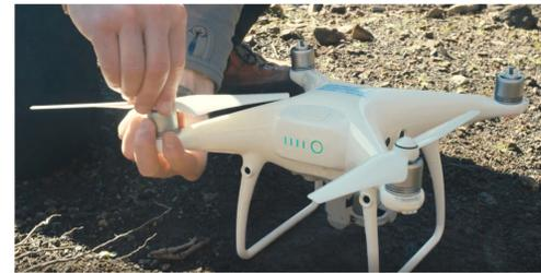
Figure 4: Quad-copter UAV used for post-landslide surveys.
