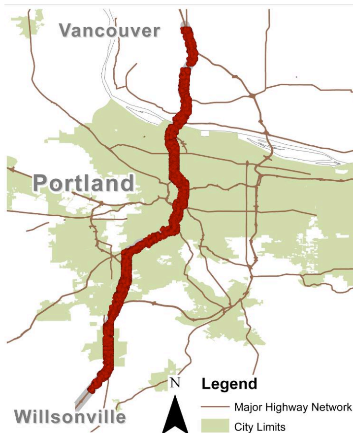
Figure 4: Map showing truck GPS data coverage provided by ATRI—individual readings on I-5 for August 2007 are shown (146,290 readings). An average of 126,000 readings occurred each month, with roughly 1,500,000 readings total for January through December 2007.
