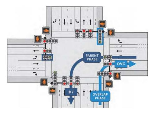
Figure 2.3: Phasing scheme for right-turn overlaps (USDOT 2015)
