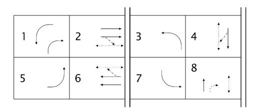
Figure 2.5: Example scheme for PPRT phasing (ODOT 2015)
