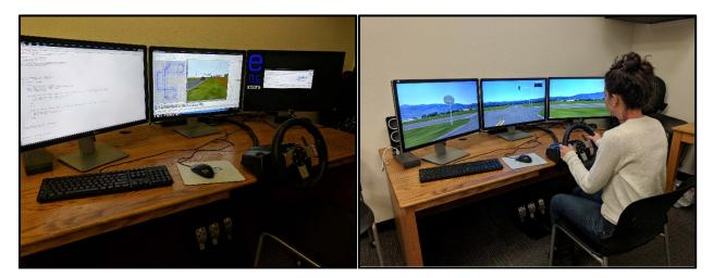
Figure 6.1: Operator workstation for driving simulator. Left: Designing an experiment in the Internet Scene Assembler with Javascript. Right: Researcher evaluating a newly designed environment
