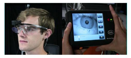
Figure 6.5: OSU researcher demonstrating the Mobile Eye XG Glasses (left) and Mobile Recording Unit (right)
