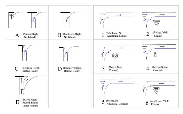
Figure 2.6: Entrance (left) and exit (right) treatments (Dixon et al. 2000)
