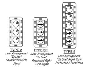
Figure 2.4 Oregon signal head types for right-turns
