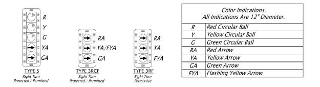
Figure 7.1: Signal Heads for Right-Turn Operations
