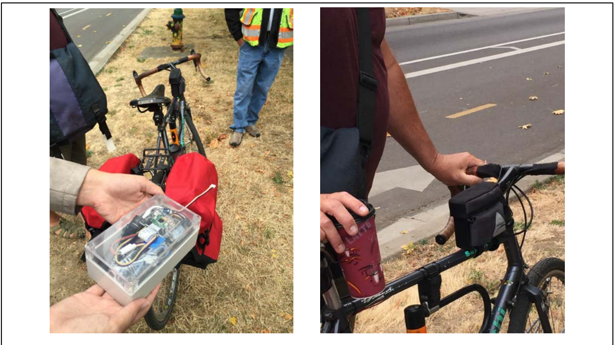
Figure 7: Prototype Bike Computer in a box and stuffed into small bike bag.
