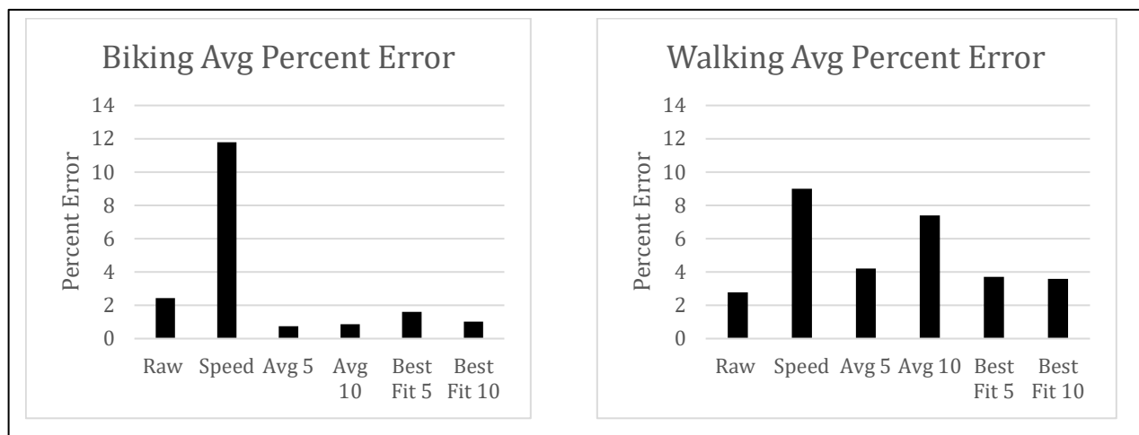
Figure 15: Percent error of the total distance traveled of biking and walking
