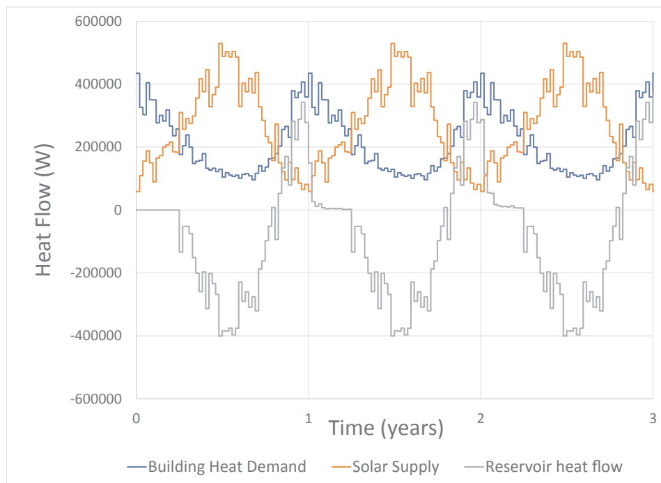
Fig. 5. Simulated heat flow components for the 125% solar/80 °C scenario (base case). Building heat load and solar heat addition are the same as from Fig. 4. RTES heat supplied is negative when surplus summer heat is injected, and positive when heat is supplied to the building from the reservoir. Heat supplied from the reservoir changes over time as the reservoir heats up.
