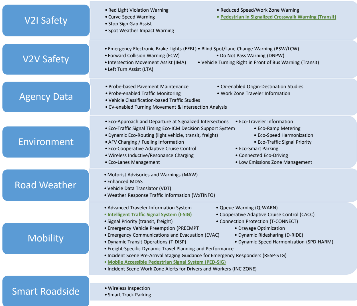
Figure 2 - U.S. DOT Connected Vehicle Applications
