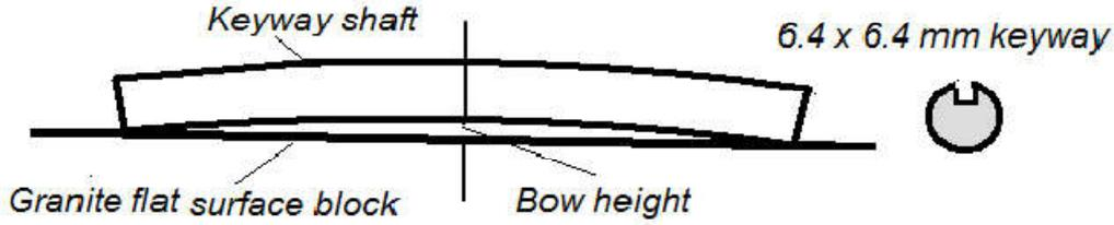
Fig. 4. Keyway shaft distortions (Kobasko, Aronov et al., 2010)
