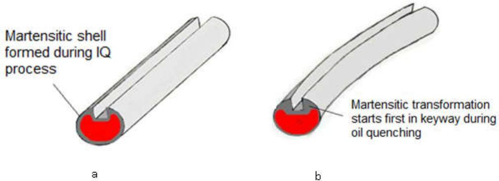
Fig. 3 Martensitic uniform shell formation in keyways during IQ process: a – providing minimum distortion due to uniform shell formation during IQ process; b – resulting in more distortion due to non-uniform shell formation during oil quenching (Table 1)
