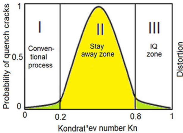
**Fig. 1. Crack formation and distortion versus Kondrat'ev number Kn (Kobasko, 1980; 2016): I – conventional processes (quenching in oil, polymers of high concentration or vacuum gas quenching); II – stay away zone; III – intensive quenching zone**
