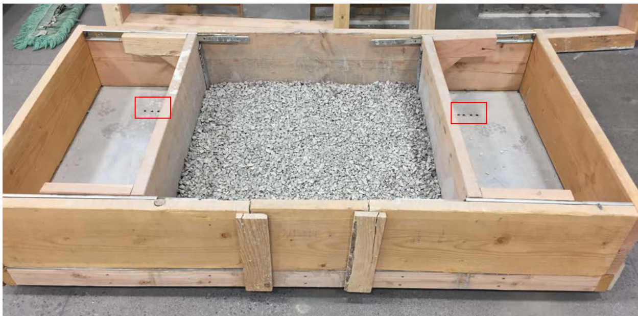
Figure 12 – Lab-scale trail testing device (red outline showing pin locations to move the walls to investigate confinement effects)
