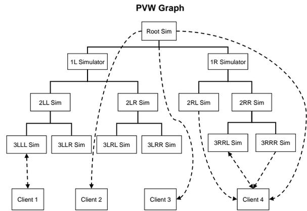
Figure 2: Network connections in a PVW instance. Dotted lines represent network connections, arrows represent information flow.
