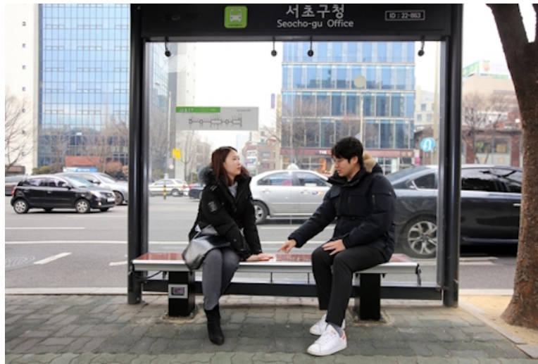
Figure 2.2. A bus stop in the Seocho District of Seoul that has a bench with heating elements to warm riders in winter months and a glass surface to cool with in the summer. Source: The Korea Bizwire.
