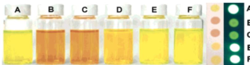
Figure 1. Color changes of fluorescein aldehyde solutions and various analytes. A) no analyte; B) L-cysteine; C) L-homocysteine; D) bovine serum albumin; E) L-glycine; F) n-propylamine. On the right, spots of fluorescein aldehyde and corresponding analytes under visible and UV light (adapted from (3)).
