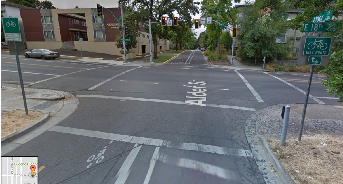
Figure 2.1: Intersection of Alder and 18th (looking south on Alder) with signal phases for bike only (left) and car only (right) and the terminal loop detector bottom left (many people on bikes wait in the crosswalk not knowing what the bike loop detector symbol is for).
