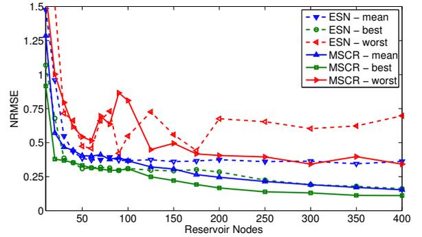
Fig. 4: NARMA performance for increasing SCR sizes. The dashed lines are obtained with regular sigmoidal neurons (ESN) and  $v = 0.01$  and  $\lambda = 0.75$ . The memristive SCR (MSCR) data was obtained based on  $v = 0.5$ ,  $\lambda = 1.7$ , and 52 memristive devices on average per node.
