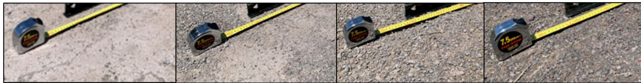
Figure 3.6: Treated surfaces (left to right: smooth, inconsistent, loose) and untreated surface (far right).
