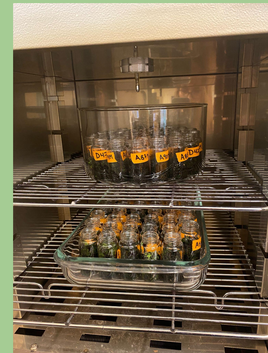
Lichen samples dehydrating in an 80°C oven for 48 hours. Samples are cooled in a desiccator.
