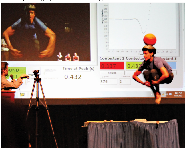
Fig. 4. Jordan Kindell, a dancer from the Oregon Ballet Theater, demonstrates how tucking in his arms and legs while jumping causes his head to deviate from a parabolic trajectory. A foam ball painted orange and attached to a bicycle helmet was used to track the position of his head during the jump. (photo courtesy AAPT).
