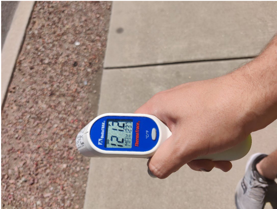
Figure 3 Delta Track ThermoTrace device being used to collect surface temperatures
