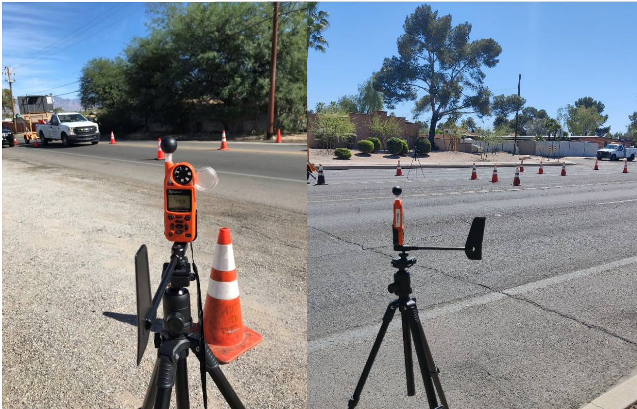
Figure 4 Kestrels placed (left) alongside the road, (right) a Kestrel between a bike lane and sidewalk and, in the distance, a Kestrel in the center lane
