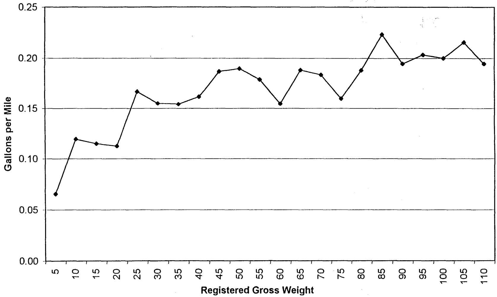
Gallons per Mile as a Function of RGW for All Truck Classes
